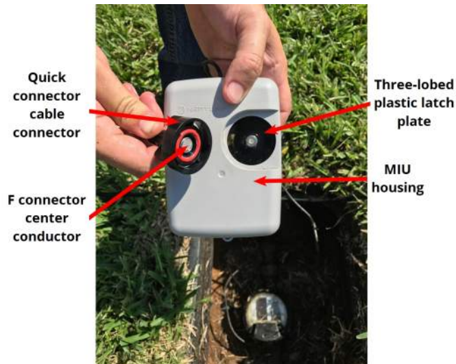
Figure 27 – Aligning the Connector to the Housing
