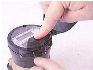
Figure 6: Placing the Cover on the Register
