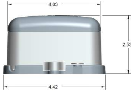
Figure 4 – Pit MIU Dimensions - Diagram 2
