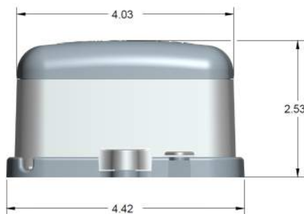
Figure 7 – Wall MIU Dimensions - Side
