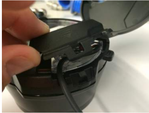
Figure 12 – Covering the Terminal Screws
