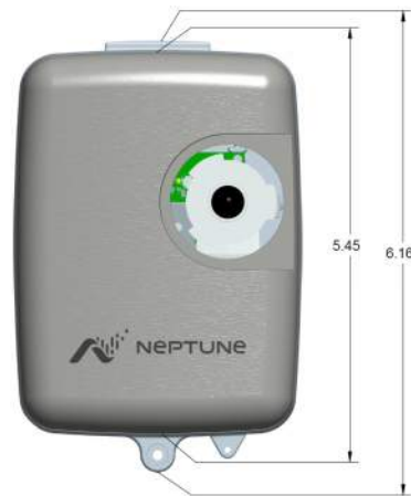
Figure 3 – Pit MIU Dimensions - Diagram 1
