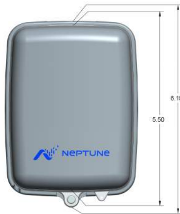
Figure 6 – Wall MIU Dimensions - Front
