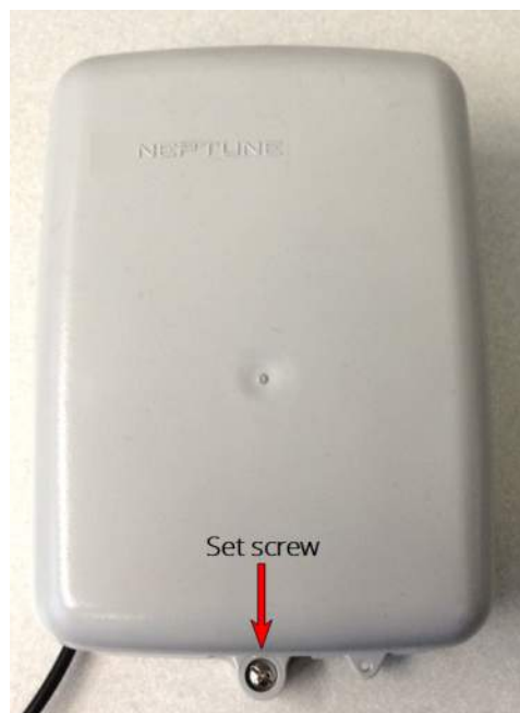
Figure 13 – Wall MIU Main Housing
