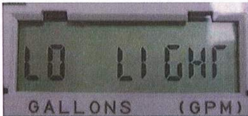
Figure 20: LCD Displays LO Light
