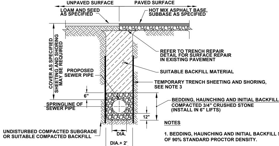
1. BEDDING, HAUNCHING AND INITIAL BACKFILL SHALL BE COMPACTED TO A MINIMUM
