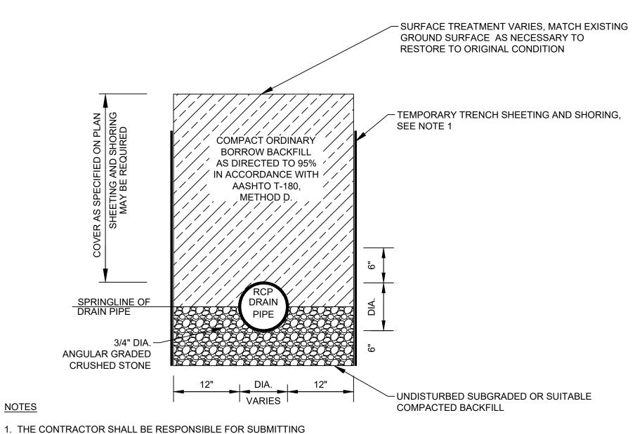
RCP DRAINAGE PIPE TRENCH DETAIL
